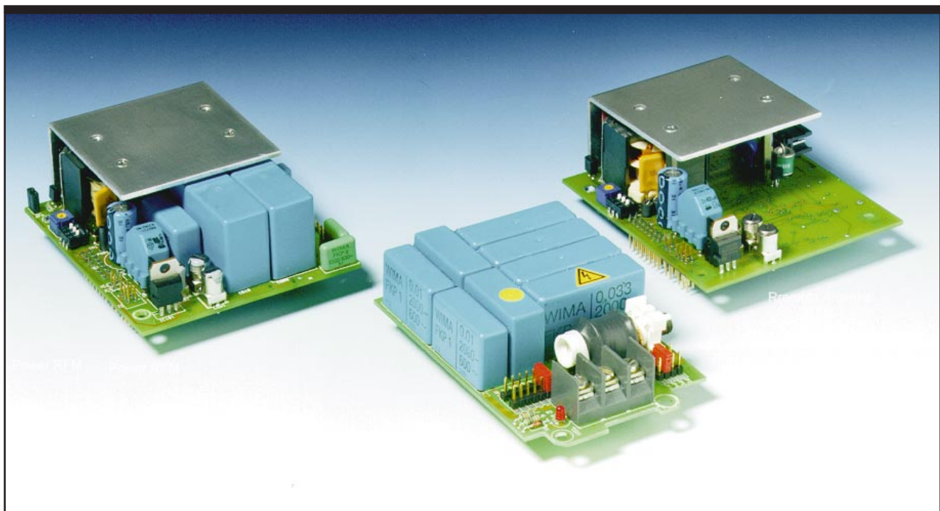
left-to-right: Standard RFM, Antenna Tuning Module, Remote Antenna RFM.
